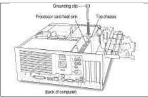
Installing the grounding clip
